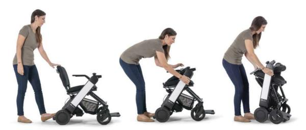
\*\*Weight is 26.7 kg. if battery is not removed. Battery weighs 2.7 kg. Note: Driving range of 20 km will vary due to user weight, drive surface, terrain, ambient temperature, speed setting, and battery charge and condition.
